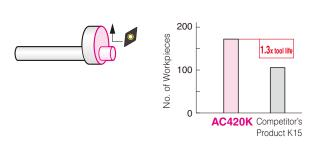
Insert: DNMG150412N-GZ (AC420K) Cutting Conditions:  $v_c$ =100 to 270m/min, f=0.15 to 0.40mm/rev,  $a_p$ =1.5mm, Wet
