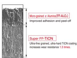
Coating stress control technology reduces abnormal damage caused by chipping.
