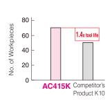
Insert: WNMA080412 (AC415K) Cutting Conditions:  $v_c$ =450m/min, f=0.25mm/rev,  $a_p$ = Up to 1.5mm, Dry
