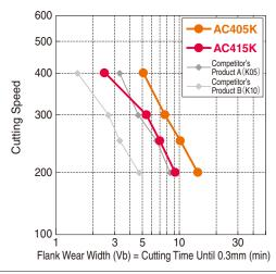
Work Material : FCD450(Round Bar) Insert : CNMG120408N-GZ Cutting Conditions:  $v_c$ =200 to 400m/min f=0.30mm/rev  $a_o$ =1.5mm Wet
