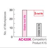
Insert: WNMA080408 (AC420K) Cutting Conditions:  $v_c$ =100 to 250m/min, f=0.15 to 0.30mm/rev,  $a_p$ =1.0mm, Wet Insert: WNMA080412 (AC420K) Cutting Conditions:  $v_c$ =200m/min, f=0.32mm/rev,  $a_p$ =3.0mm, Wet
