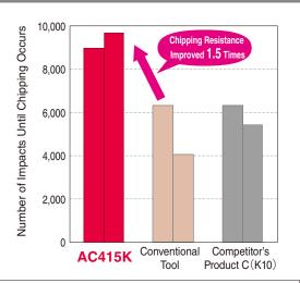
Work Material : FCD450 Insert : CNMG120408N-GZ Cutting Conditions: v<sub>c</sub>=300m/min f=0.25mm/rev
