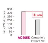
Insert: CNMG120408N-UZ (AC405K) Cutting Conditions: v<sub>c</sub>=300m/min, f=0.20mm/rev, a<sub>p</sub>=0.5mm, Wet
