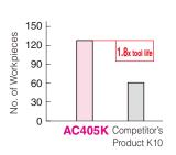
Insert: DNMG150408N-UZ (AC405K) Cutting Conditions:  $v_c$ =200m/min, f=0.45mm/rev,  $a_p$ =0.25 to 0.40mm, Wet
