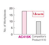
Insert: CNMA120408 (AC415K) Cutting Conditions:  $v_c$ =230m/min, f=0.2 to 0.3mm/rev,  $a_p$ =1.5 to 2.0mm, Wet Insert: WNMA080412 (AC415K) Cutting Conditions:  $v_c$ =230m/min, f=0.30mm/rev,  $a_p$ =1.5 to 2.5mm, Dry
