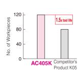
Insert: CNMG120412N-GZ (AC405K) Cutting Conditions:  $v_c$ =500m/min, f=0.25mm/rev, Up to  $a_p$ = to 2.0mm, Dry
