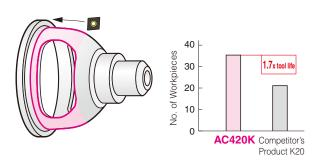
Insert: CNMA120408 (AC420K) Cutting Conditions:  $v_c$ =250m/min, f=0.30mm/rev,  $a_p$ =2.0 to 3.0mm, Wet
