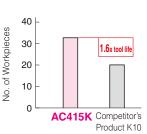
Insert: CNMG120408N-GZ (AC415K) Cutting Conditions: v<sub>c</sub>=240m/min, f=0.3mm/rev, a<sub>p</sub>=2.0 to 3.0mm, Wet
