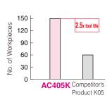
Insert: WNMG080408N-UZ (AC405K) Cutting Conditions: v<sub>c</sub>=340m/min, f=0.3mm/rev, a<sub>p</sub>=0.2mm, Wet
